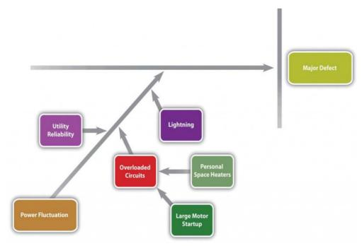
Figure 14.6 Possible Causes of Power Fluctuation
