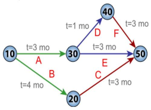
Figure 1.4 Pert Chart by Jeremykemp derivative work: Hazmat2 from Wikimedia Commons
